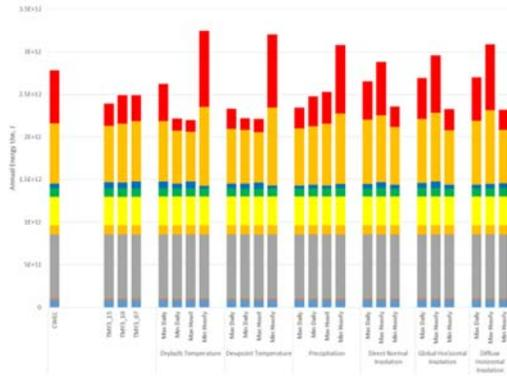
Figure 13. TMY and XMY Energy End-Uses for Medium Office, Yellowknife
