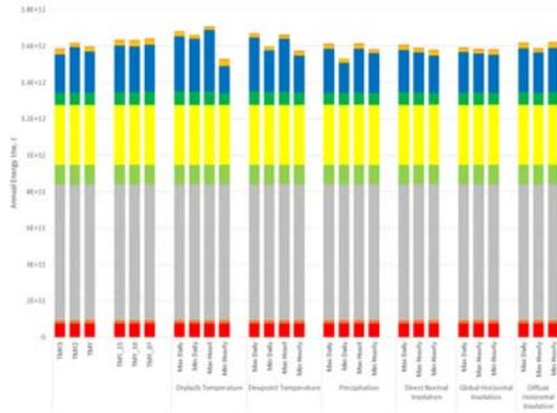
Figure 12. TMY and XMY Energy End-Uses for Medium Office, San Diego
