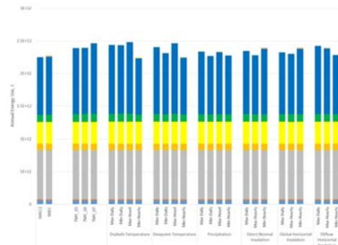
Figure 11. TMY and XMY Energy End-Uses for Medium Office, Dubai
