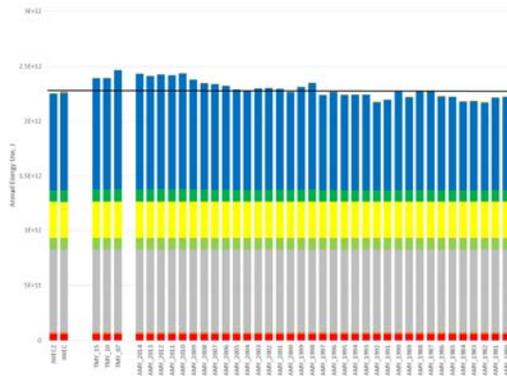
Figure 14. TMY and AMY Energy End-Uses for Medium Office, Dubai
