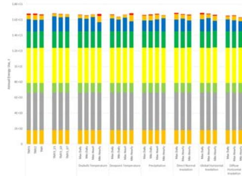
Figure 8. TMY and XMY Energy End-Uses for Small Office, Washington Dulles
