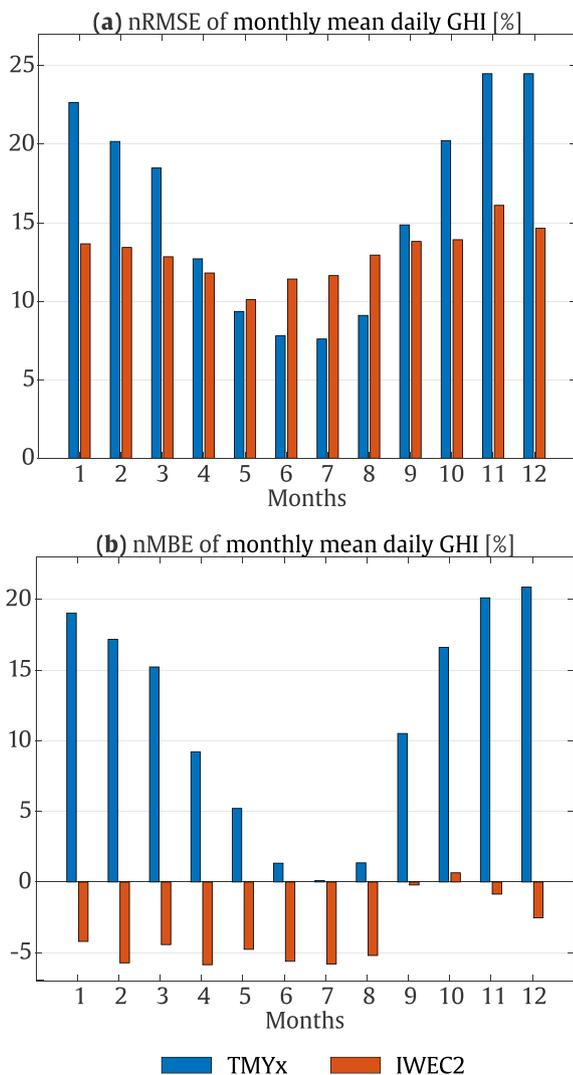
**Fig. 5.** Error bar plot of the radiation modeling approaches through the monthly mean daily GHI index for the TMYs derived from the period 2003–2017. (a) nRMSE; (b) nMBE.
