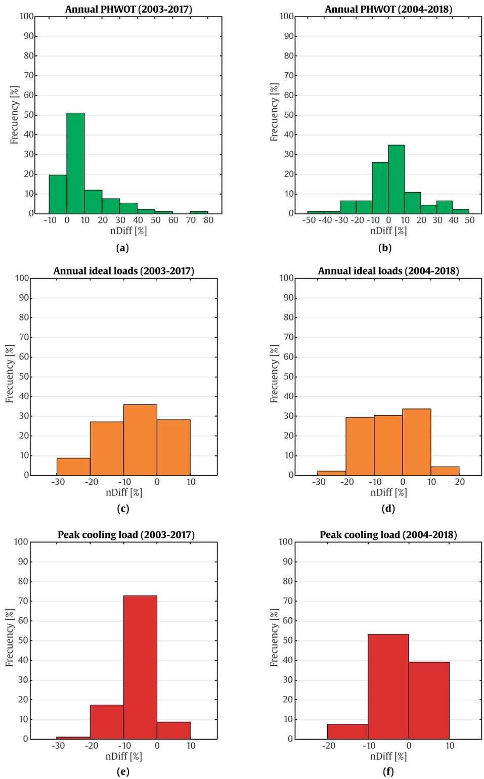
**Fig. 21.** nDiff distribution of the reference residential building driven only by a change of solar radiation modeling in both original databases (TMYx.2003–2017 and TMYx.2004–2018).
