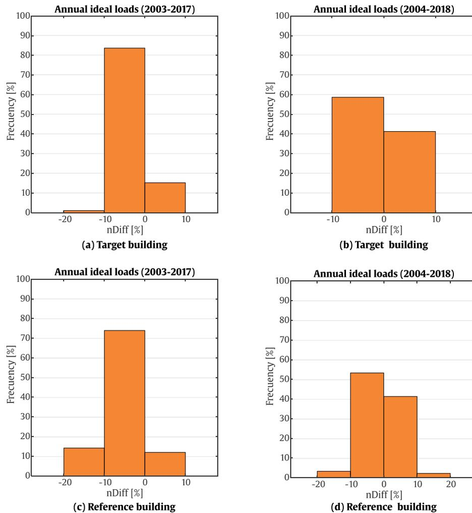
Fig. 22. nDiff distribution of annual ideal loads for the target commercial building and its reference model driven only by a change of solar radiation modeling in both original databases (TMYx.2003–2017 and TMYx.2004–2018).
