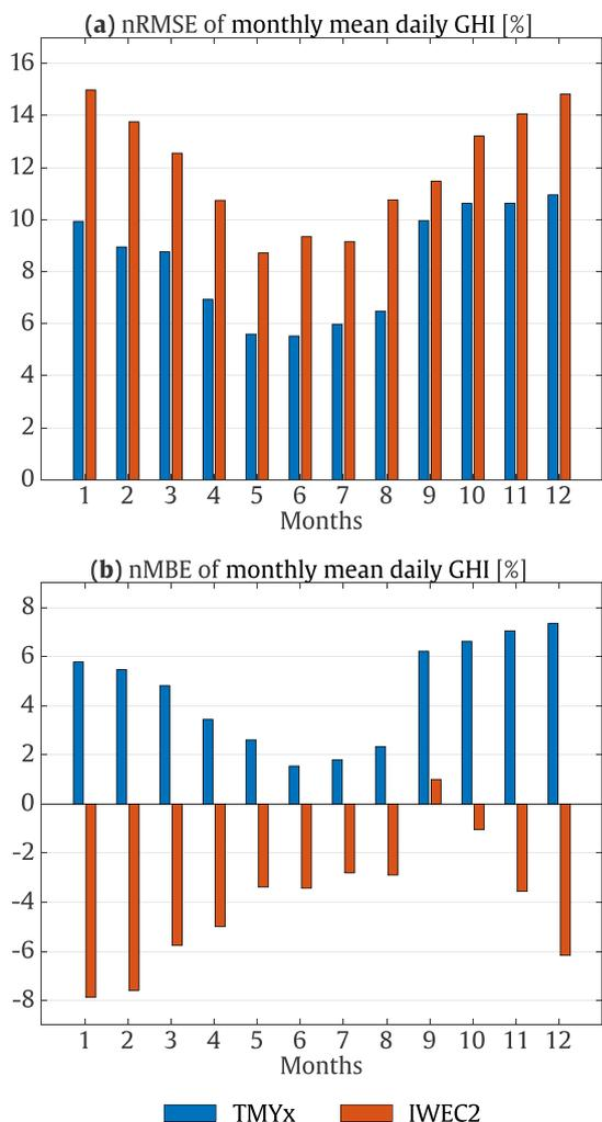
Fig. 8. Error bar plot of the radiation modeling approaches through the monthly mean daily GHI index for the TMYs derived from the period 2004–2018. (a) nRMSE; (b) nMBE.
