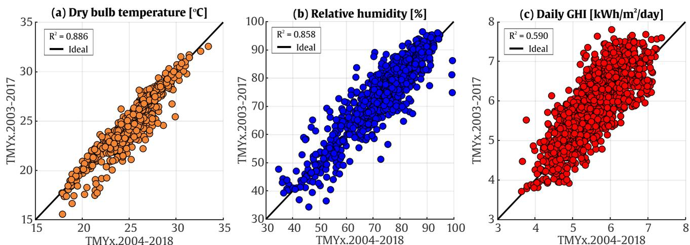
Fig. 15. Correlation between the resulting monthly mean values of the primary variables in the TMYx.2003–2017 and TMYx.2004–2018 databases, which are used to determine the TMYs in ISO 15927–4:2005 method. (a) Monthly mean dry bulb temperature; (b) Monthly mean relative humidity; (c) Monthly mean daily GHI.
