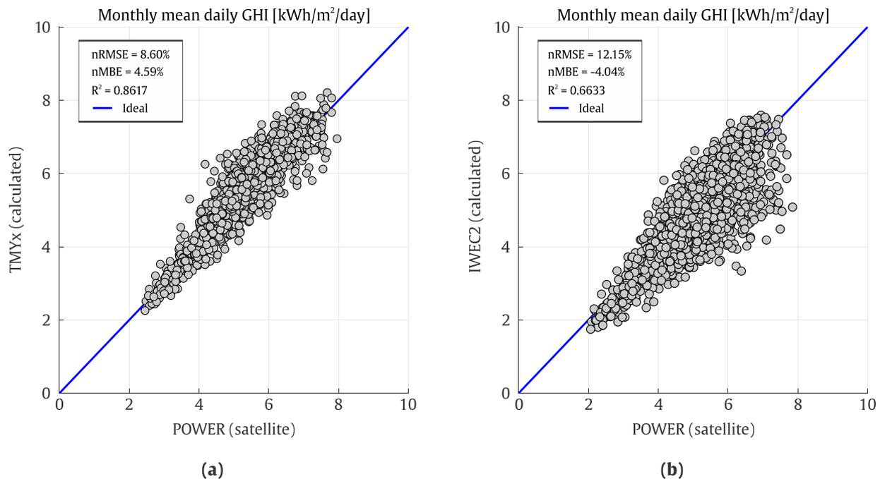
**Fig. 7.** Comparison, using monthly mean daily GHI index, of calculated solar radiation against the satellite derived (POWER) ones for the TMXs derived from the period 2004–2018. (a) TMX models (IWEC approach). (b) IWEC2 approach.
