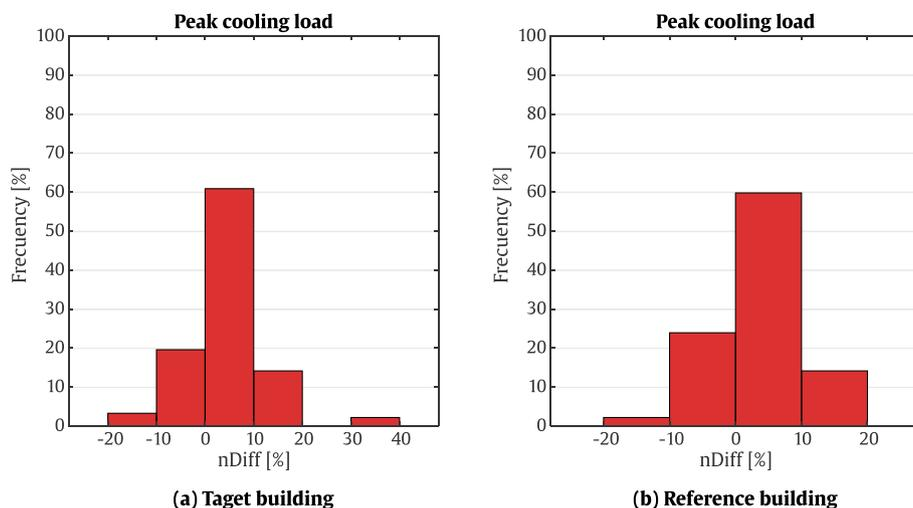
Fig. 18. nDiff of the peak cooling loads for the residential buildings obtained by using both databases, TMYx.2003–2017 and TMYx.2004–2018, in 92 Brazilian locations.
