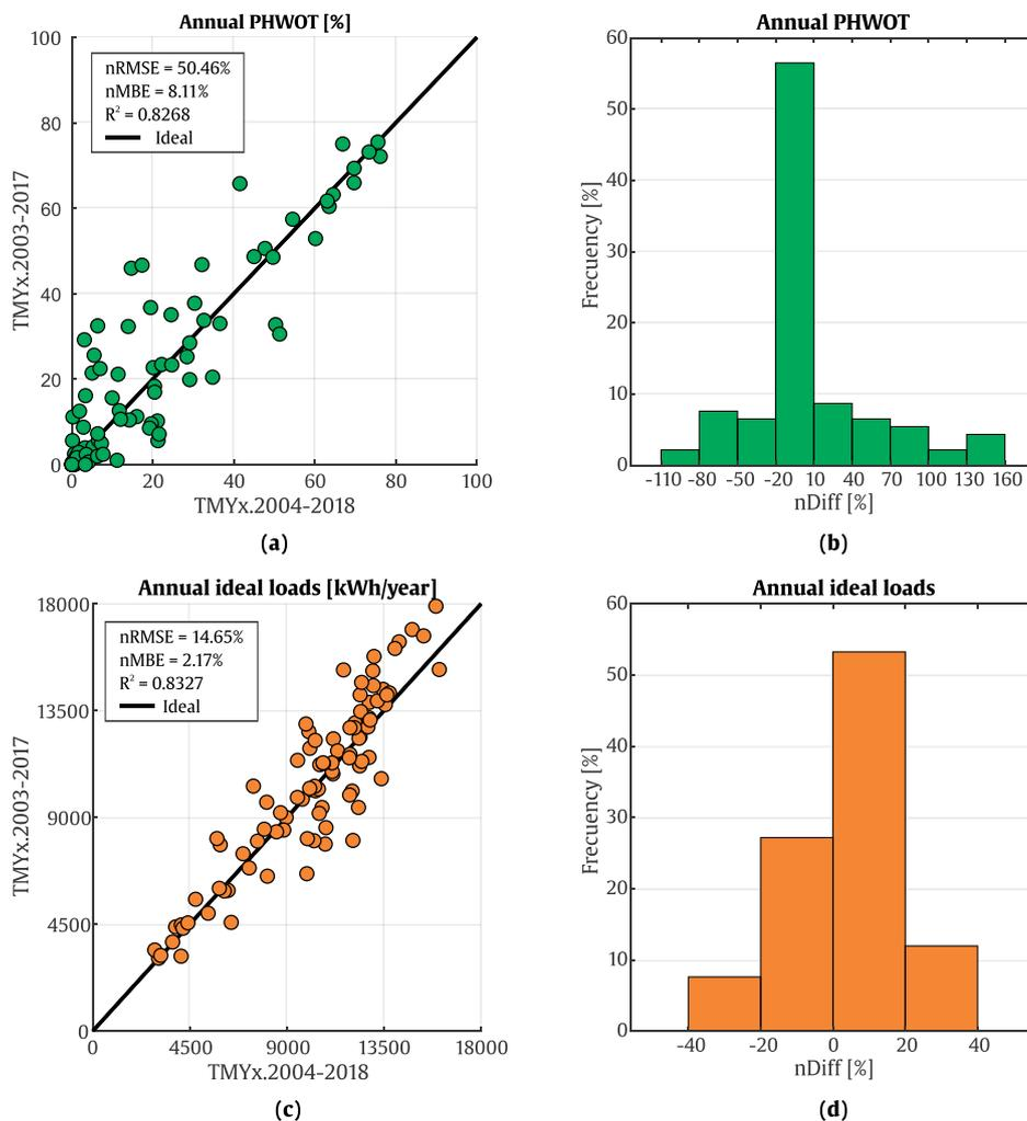
Fig. 17. Comparison of annual BPS results for the reference model of the residential building obtained by both databases TMYx.2003–2017 and TMYx.2004–2018 in 92 Brazilian locations.
