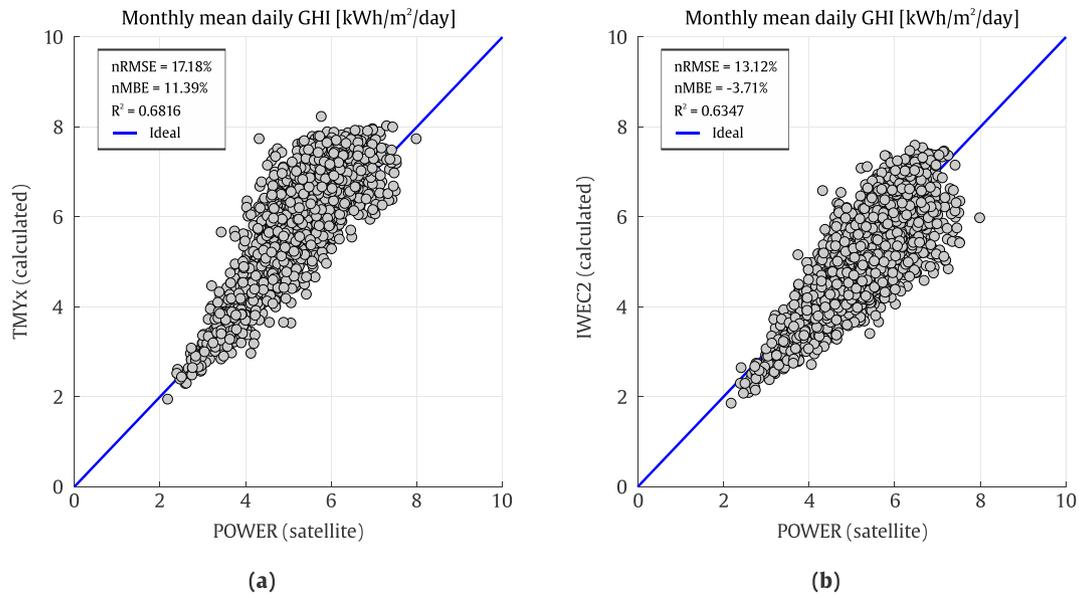
**Fig. 4.** Comparison, using monthly mean daily GHI index, of calculated solar radiation against the satellite derived (POWER) ones for the TMYs derived from the period 2003–2017. (a) TMYx models (IWEC approach). (b) IWEC2 approach.
