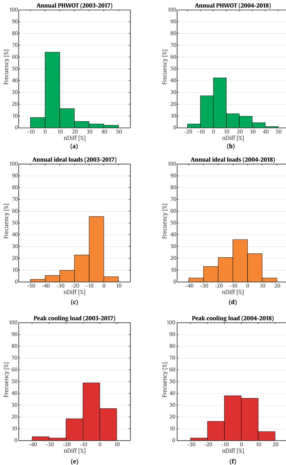
**Fig. 20.** nDiff distribution of the target residential building driven only by a change of solar radiation modeling in both original databases (TMYx.2003–2017 and TMYx.2004–2018).
