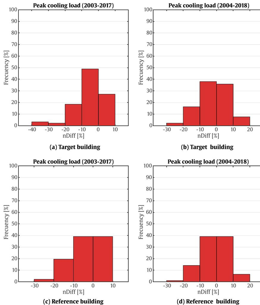
**Fig. 23.** nDiff distribution of peak loads for cooling in the target commercial building and its reference model driven only by a change of solar radiation modeling in both original databases (TMYx.2003–2017 and TMYx.2004–2018).
